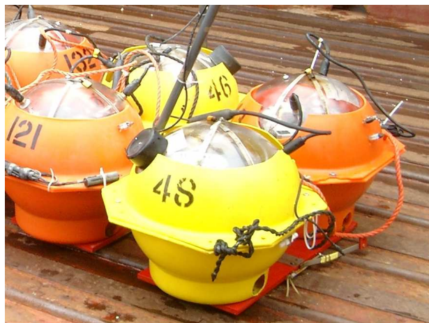
Figure 11: The GeoPro type OBS with two glass spheres, one for the releaser unit and the other for the seismometer unit.
