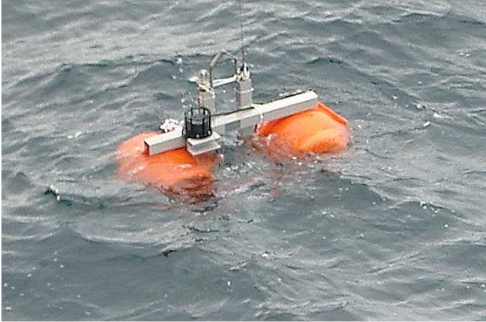
Figure 10: The Hamburg type OBH with two glass spheres covered by orange plastic, which are mounted on a GFK frame. The datalogger is stored in the red pressure cylinder made of aluminium. The silver aluminium housing covers the hydrophone.
