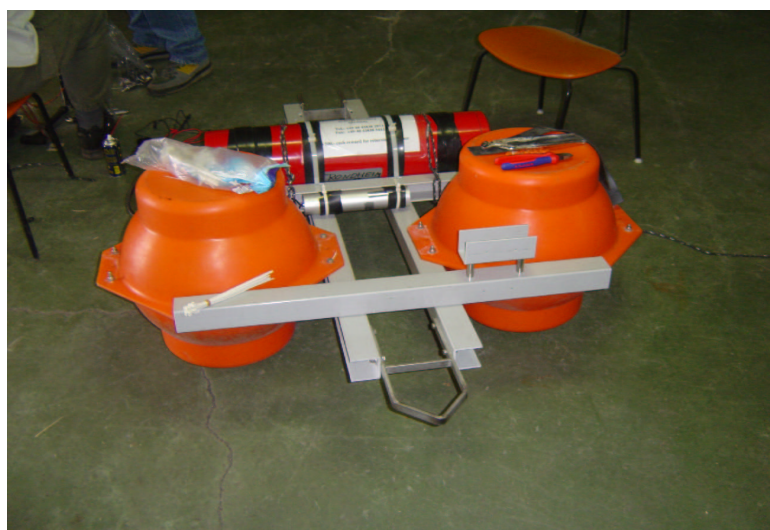
Figure 13: The Hamburg type OBH with two glass bowl covered by orange plastic, which are mounted on a GFK frame. The datalogger is stored in the red pressure cylinder made of aluminium. The silver aluminium housing covers the hydrophone.
